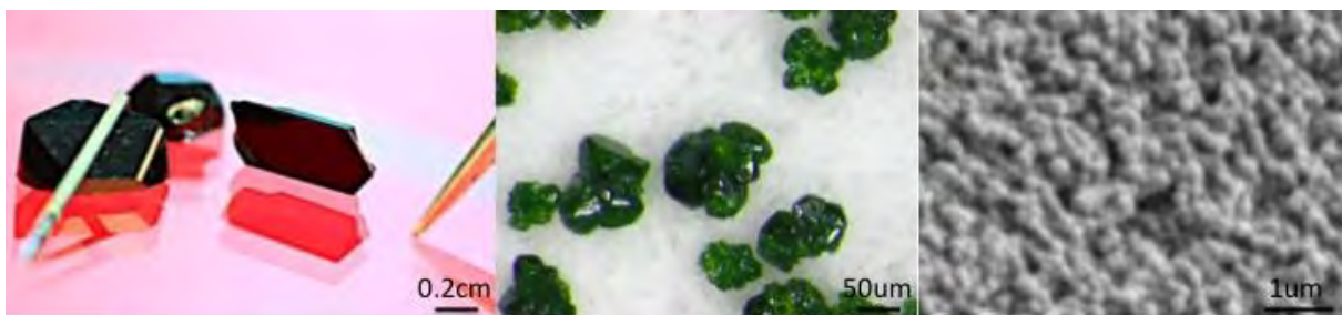
Figure 1: \text{Cu}_2\text{OSeO}_3 crystals grown by Chemical Vapor Transport (left), grown by hydrothermal process (center and right).
